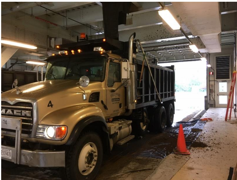
Figure WTR-2. Post-centrifuge WTRs being loaded onto contractor trucks to haul away for land application
