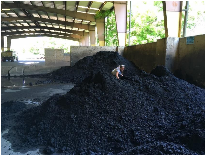
Figure WTR-4. Stockpiled WTRs awaiting transport, which allows for some extra drying time
